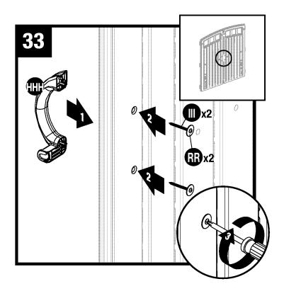
Attach door handle (HHH) to left door with two screws (III) and two washers (RR). Repeat for right door.
