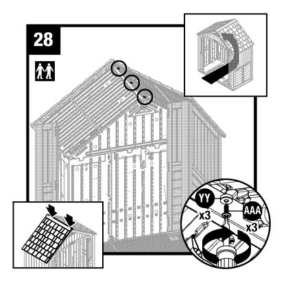
Push down the roof from outside. From inside shed, secure roof panels together along ridge of roof using three rubber washers (YY) and three sealing screws (AAA).
