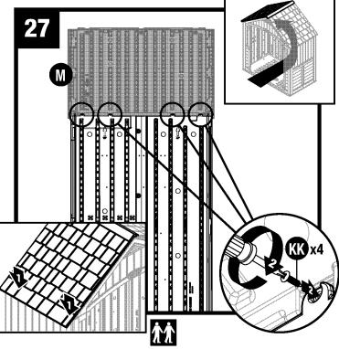
Pull down each lower corner of left roof (M) from outside. From inside shed, attach each tab to the corresponding roof panel with one screw (KK).
