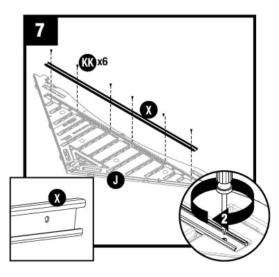
Lay front header (J) on ground with lettering side facing up. Place one header beam (X) into pocket on inside of front header. Attach with six screws (KK). **DO NOT** over tighten screws.
