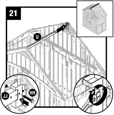
Raise ridge beam (U) up and into rear roof ridge beam bracket. Secure with one 2" hex bolt (HH) and one nut (JJ).
