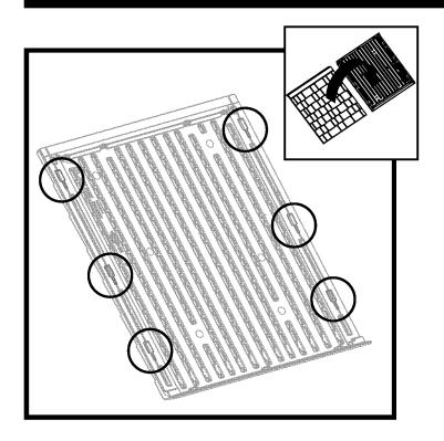
Before proceeding, locate and identify six dovetails on interior side of right roof (L) and left roof (M).
