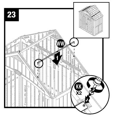
Attach roof support bracket (WW) to front and rear headers. Secure with two screws (KK).
