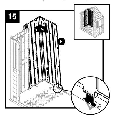
Tip back corner (E) back to vertical position and align lower tabs on left side with slots in floor.
