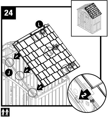
Lay right roof (L) directly over three tabs on right side of front header (J). With right roof slots seated over/on header tabs, check alignment in all three spots. Slide right roof (L) down towards the outside of shed. You will hear a "snap" when engaged.
