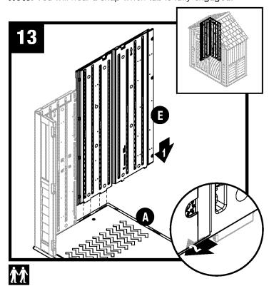
Align tab on bottom left side of back corner (E) with slot on front floor (A). Lower panel into slot and lock in place by sliding panel toward front corner.
