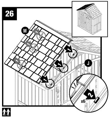
Lay left roof (M) directly over the three tabs on left side of front header (J). With left roof slots seated over/on header tabs, check alignment in all three spots. Slide left roof (M) down towards the outside of shed. You will hear a "snap" when engaged.
