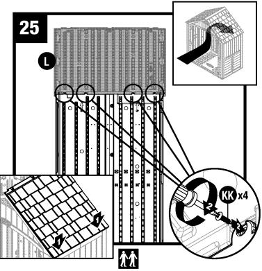
Pull down each lower corner of right roof (L) from outside. From inside shed, attach each tab to the corresponding roof panel with one screw (KK).
