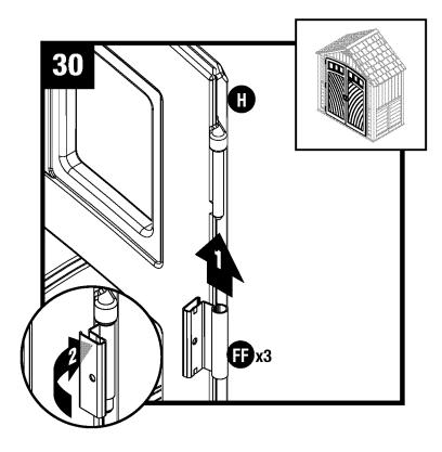
Stand right door (H) upright with three hinge mounts facing right. Slide one metal hinge plate (FF) up onto each hinge mount. Rotate hinge plates to outside of door.
