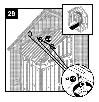
Secure roof support bar to roof using three screws (KK). Repeat for remaining roof support bar (WW).
