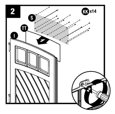
Stand left door (I) vertically. In this order, layer into door channel the window gasket (TT), and door window (S). Through the back of door, secure layers with fourteen screws (KK). Start with four corner screws and finish with remaining screws. **DO NOT** over tighten screws.
