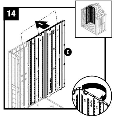
Tip back corner (E) outward slightly and bend corner hinge.
