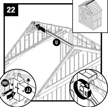
Slide ridge beam (U) into front roof ridge beam bracket. Secure with one 2" hex bolt (HH) and one nut (JJ).
