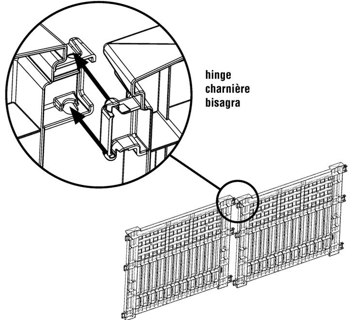
2. Stand fence upright. On the back side of fence, unsnap stakes and swing toward center of panel. Pull up to remove.
