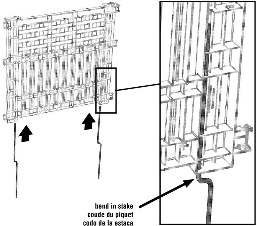
4. Position fence in desired location. Using a mallet, tap stakes at the bend until the bend is tapped down to the ground.
